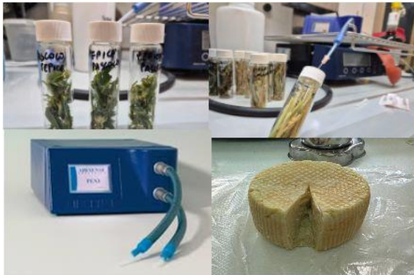
Figure 1 - Objective olfactory assessment with electronic nose
