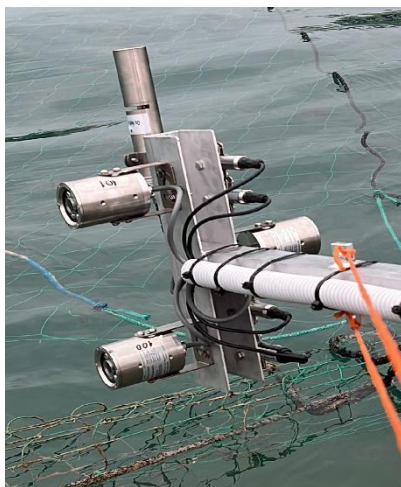
Figure 1 - Video monitoring system - Position of the 3 underwater cameras on the monitoring bracket in the farming cage.
