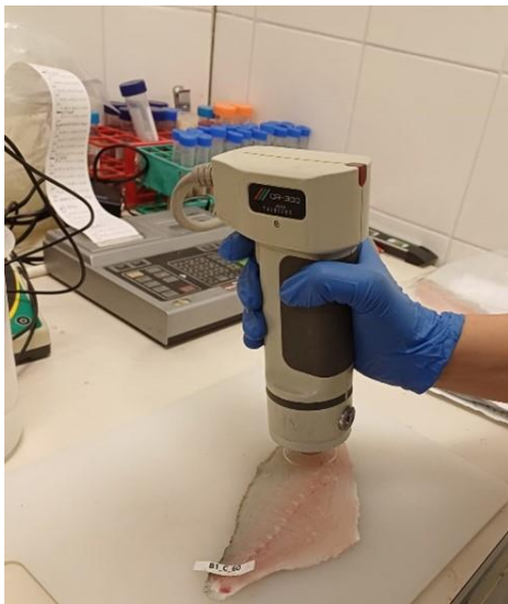
Figure 1 – Colour analysis of the fish fillet
