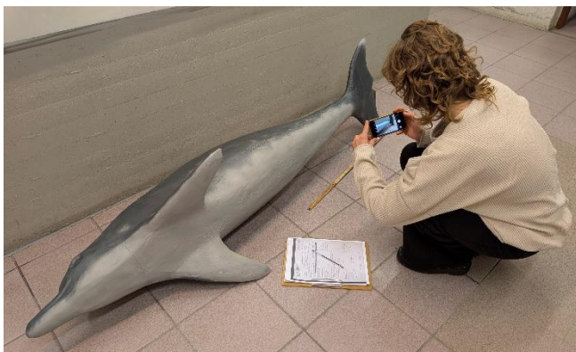
Figure 1 – First 1:1 (184cm long) 3D printed dolphin produced as a proof of concept.
